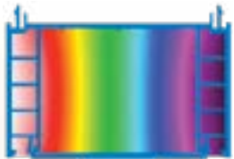
Thermographic cross-section of a 50 mm StyroClick extension profile.
