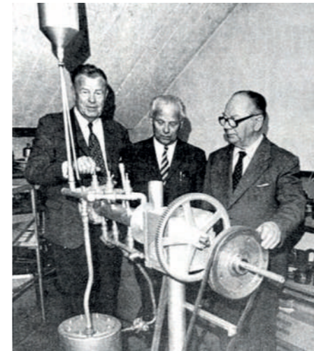
Norwegian Extruding founder Johan Aasheim (front) transformed a meat grinder into the first extruder in the Nordic region. Here he is photographed with Extruder 1.
