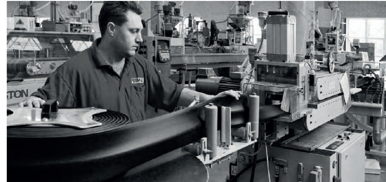
Plastic sealing being reeled into big rolls immediately after being extruded.
