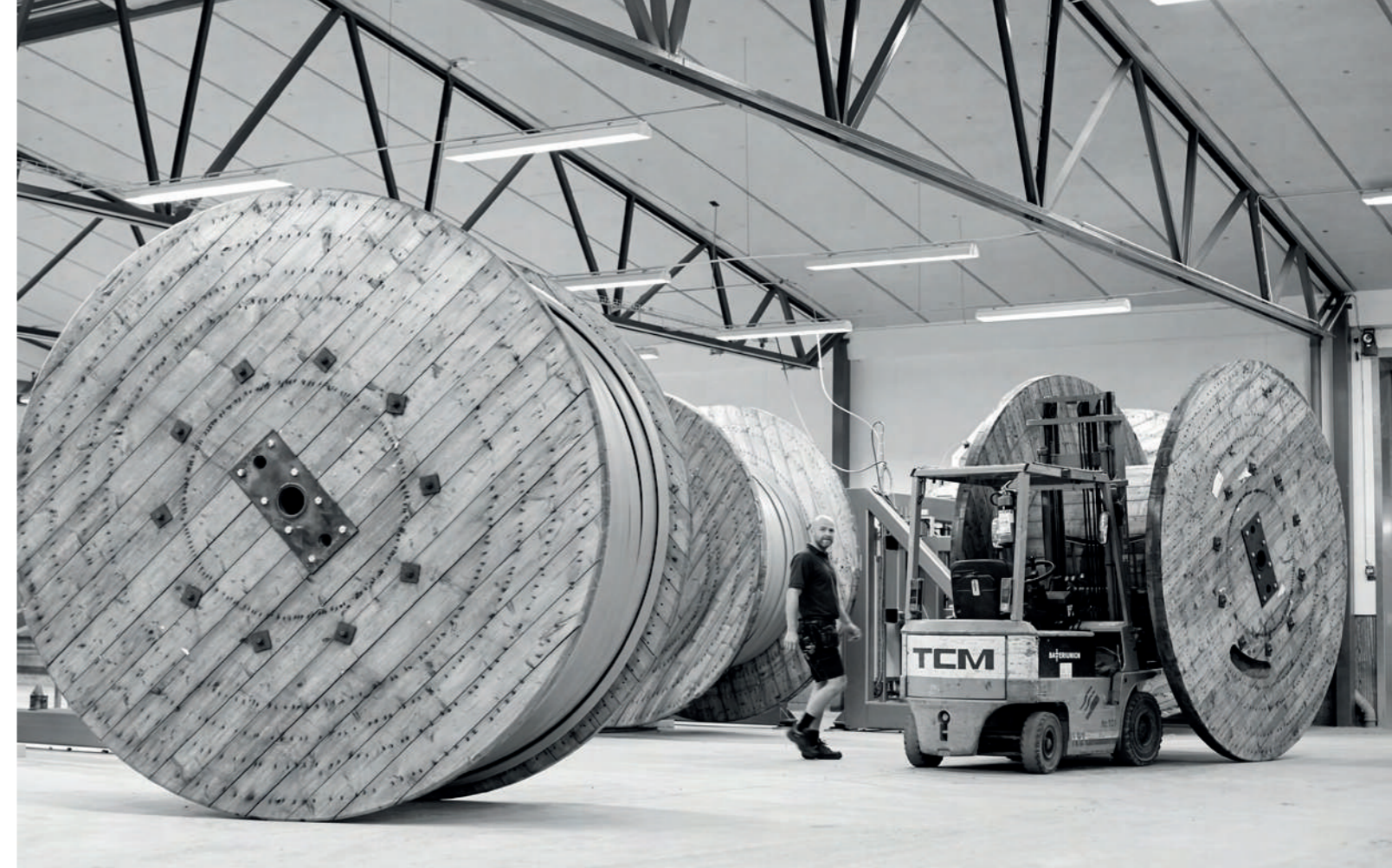
Fillers and rods for offshore cables are rolled onto large cable reels that are stored until the customer needs them.
