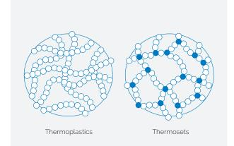
Thermoplastics can be remelted (plasticised) and processed again several times, generally without losing their properties, which also make them convenient for recycling. Thermoplastics is the most common type utilized in extrusion processes and people often associate the attributes of thermoplastic, when they think of "plastic"
