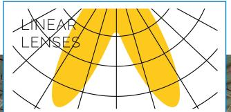
Linear lens profiles are used to create special lighting patterns with highest efficiency and protect the light source at the same time.
